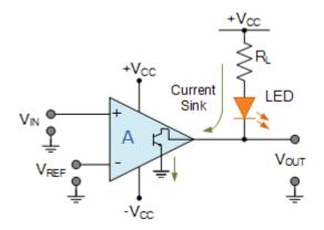
Here, the open collector output from the voltage comparator is connected to a voltage source via a single pull-up resistor (and an LED for indication) which pulls the single output high to the power supply. When the output switch is HIGH it creates a high impedance path, therefore no current flows as  $V_{OUT} = Vcc$ .
