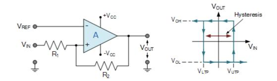
Note that the arrows on the hysteresis graph indicate the direction of switching at the upper and lower trip points.
