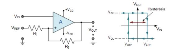
For the inverting comparator circuit above,  $V_{IN}$  is applied to the inverting input of the op-amp. Resistors  $R_1$  and  $R_2$  form a voltage divider network across the comparator providing the positive feedback with part of the output voltage appearing at the non-inverting input. The amount of feedback is determined by the resistive ratio of the two resistors used and which is given as:
