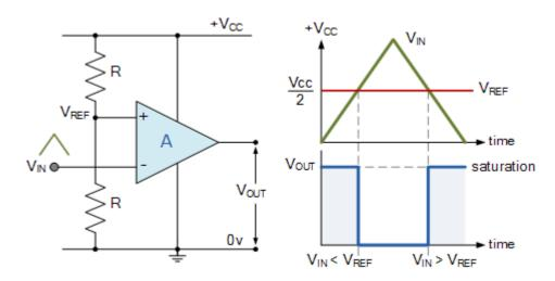
In the inverting configuration, which is the opposite of the positive configuration above, the reference voltage is connected to the non-inverting input of the operational amplifier while the input signal is connected to the inverting input. Then when  $V_{\rm IN}$  is less than  $V_{\rm REF}$  the op-amp
