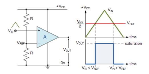
In this non-inverting configuration, the reference voltage is connected to the inverting input of the operational amplifier with the input signal connected to the non-inverting input. To keep things simple, we have assumed that the two resistors forming the potential divider network are equal and: R1 = R2 = R. This will produce a fixed reference voltage which is one half that of the supply voltage, that is Vcc/2, while the input voltage is variable from zero to the supply voltage.
