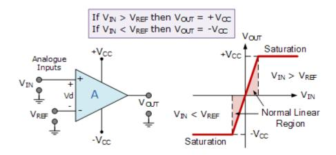
With reference to the op-amp comparator circuit above, lets first assume that  $V_{IN}$  is less than the DC voltage level at  $V_{REF}$ , ( $V_{IN} < V_{REF}$ ). As the non-inverting (positive) input of the comparator is less than the inverting (negative) input, the output will be LOW and at the negative supply voltage, -Vccresulting in a negative saturation of the output.
