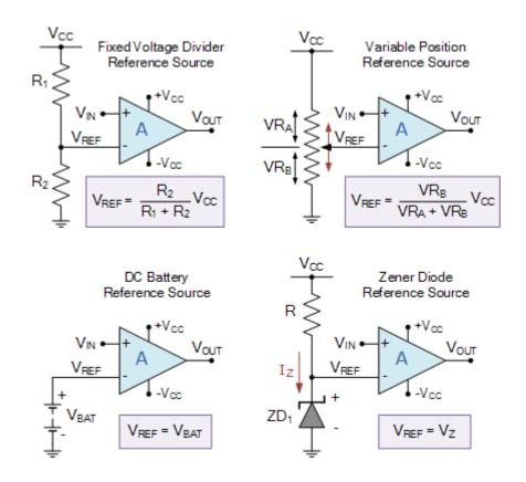
In theory the comparators reference voltage can be set to be anywhere between 0v and the supply voltage but there are practical limitations on the actual voltage range depending on the op-amp comparator being device used.
