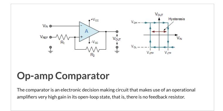
The **Op-amp comparator** compares one analogue voltage level with another analogue voltage level, or some preset reference voltage,  $V_{REF}$  and produces an output signal based on this voltage comparison. In other words, the op-amp voltage comparator compares the magnitudes of two voltage inputs and determines which is the largest of the two.
