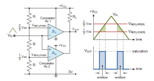
When  $V_{\rm IN}$  is below the lower voltage level,  $V_{\rm REF(LOWER)}$  which equates to 1/3Vcc, the output will be LOW. When  $V_{\rm IN}$  exceeds this 1/3Vcc lower voltage level, the first op-amp comparator detects this and switches the output HIGH to Vcc.
