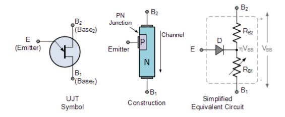
Notice that the symbol for the unijunction transistor looks very similar to that of the junction field effect transistor or JFET, except that it has a bent arrow representing the Emitter(E) input. While similar in respect of their ohmic channels, JFET's and UJT's operate very differently and should not be confused.
