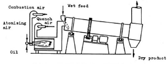
Typical cascading direct rotary dryer arranged for cocurrent operation. (From Nonhebel and Moss, 1971.)
