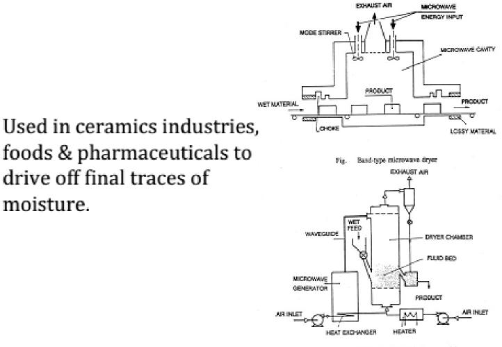
Fig. Microwave dryer for particulate materials
