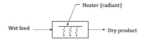
Vacuum or low gas flow to carry evaporated moisture away.
