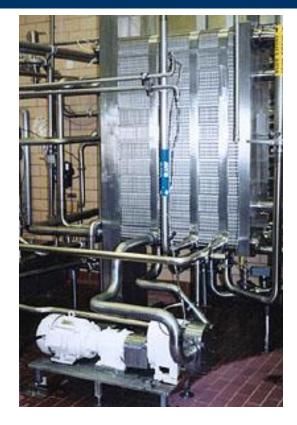
Defined as: "The heating of every particle of milk or milk product to a specific temperature for a specified period of time without allowing recontamination of that milk or milk product during the heat treatment process."
